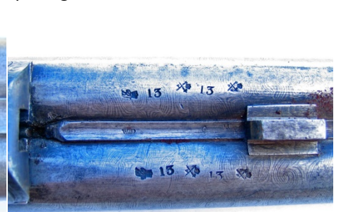
By refitting the pin fire hammers this gun can be used with pin fire cartridges. Birmingham private proof marks.
