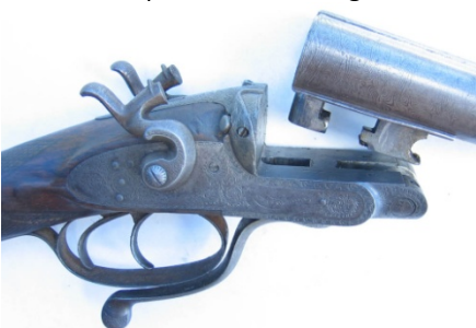
Under lever barrel locking detail.
