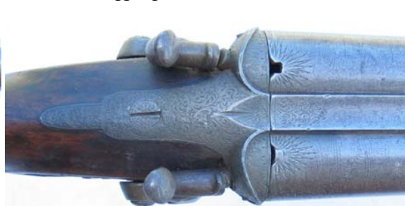
By refitting the pin fire hammers this gun can be used with pin fire cartridges. Birmingham private proof marks.
