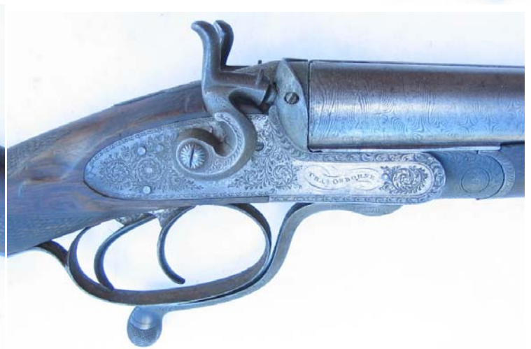
None rebounding hammers, side locks and barrel easily removed for cleaning & servicing.
